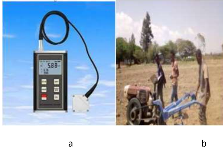
Figure 2. (a) VM-6380 3-Axis 3D Digital Vibration Meter Tester. (b) Field measurement of vibration characteristics.
