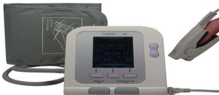
Figure 4. Finger Pulse Oximeter with digital blood pressure monitor (Contec Medical Systems Co., Ltd. China).
